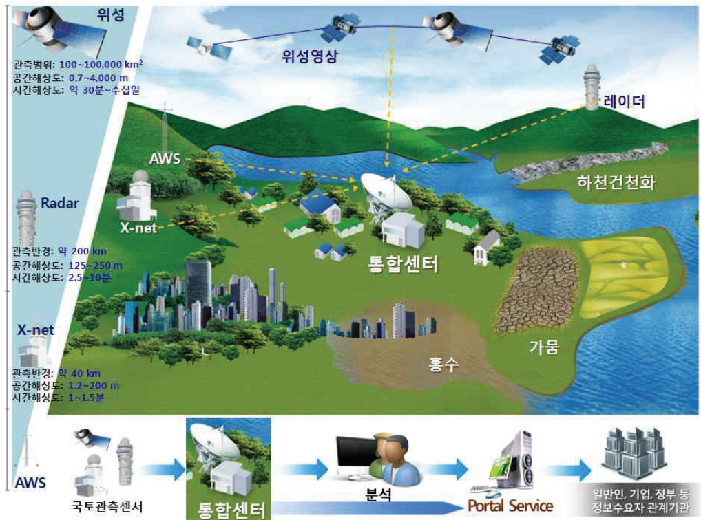
Figure 4. Flood Monitoring System using SRA
