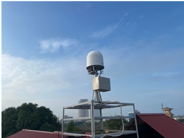
The EAGLE radar is a new meteorological radar that performs 3D observation of 50-km periphery in 30 seconds.
